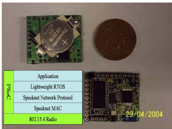
Figure 2. The Speck prototype “ProSpeckz” and its system overview diagram
